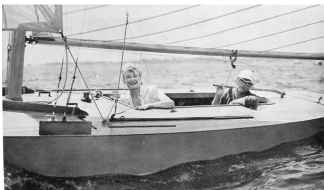
George & Juanita Elder in ISCYRA VI in 1941 Items of note: massive mast; mechanical mast partners; roller reefing with "claws"; fixed gooseneck; below-deck halyard cleating; single jib fairlead loop; long chainplates; snubbing winch.
