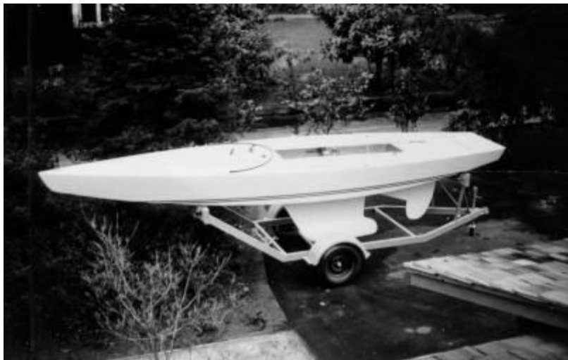
Star # 5445, Magic, built for Bob Rodgers of the Green Lake fleet. Trailer built by Spar Tech. Note the position of the traveler, half way between the rudderpost and the transom. The starboard bilge pump is just visible in the cockpit.
